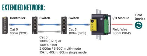
The distributed Ethernet architecture allows for enhanced connectivity and flexibility. Ethernet improves lifecycle management by enabling replacement or upgrade of individual components. The "future-proof" architecture of the Mark VIe platform enables a control system lifetime engineered to exceed expectations.
