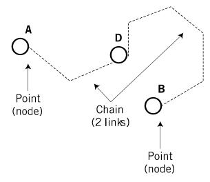
The manifold for this network would contain at least switches and cables. A rule would be defined within this manifold that automatically connects the switches to the cable (when they overlap during input). This is called a connect-split link rule in Smallworld parlance. Adding a third switch, *D*, reveals the benefit of this
