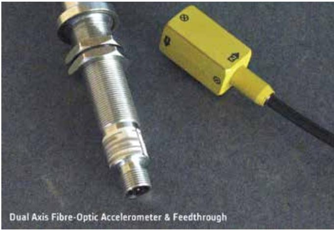
Dual Axis Fibre-Optic Accelerometer & Feedthrough
